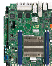
Xeon® D SoC Skylake-D Intel® Quick Assist Technology Quad 10GbE LAN Embedded
